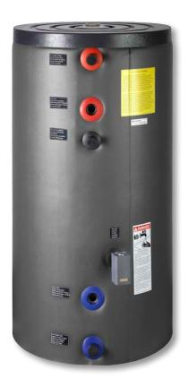
The glass lined indirect hot water heater offers an affordable solution in areas where high chloride levels in the domestic water supply can corrode a stainless steel tank. The internal coil delivers unmatched performance with a large surface area resulting in high domestic hot water ratings.
